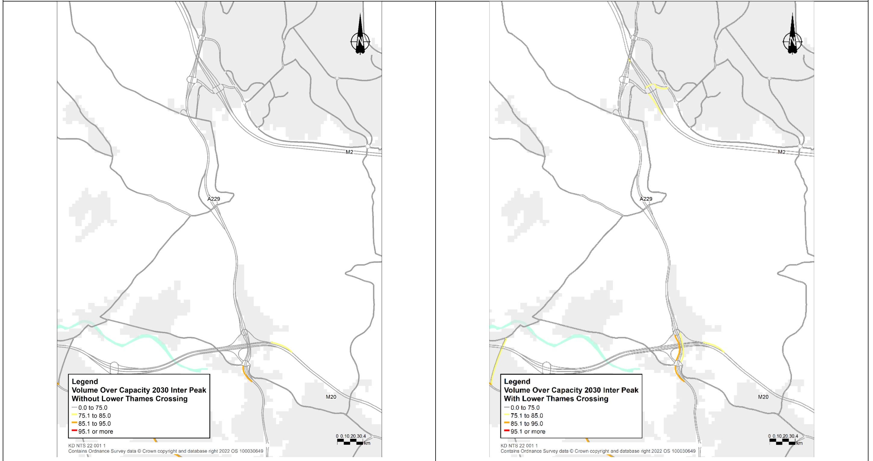
Figure A-2 – Volume over Capacity Plots for Blue Bell Hill corridor (2030, Inter-peak)
