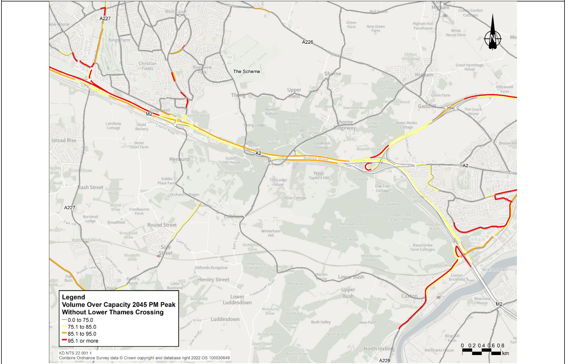
Figure A-30 – Volume over Capacity Plots for A2/M2 corridor (East) (2045, PM peak)
